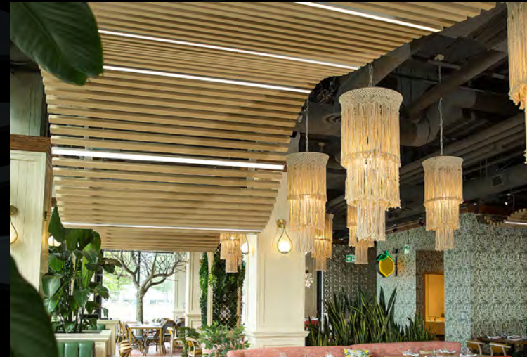
Undulating acoustic beams with integrated LED strip lighting.
